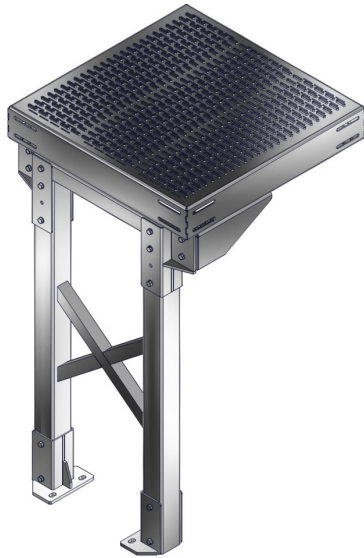
Flush bolting arrangement used when supporting one platform.
